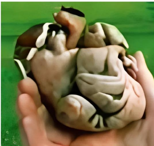
FIGURE 8: After thermal treatment MSW turn it easier to put apart PVC from other plastics.
