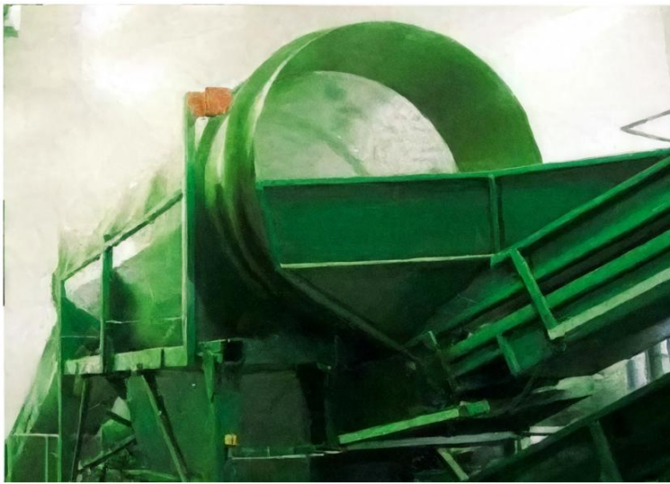
FIGURE 4: Homogenization trommel - part of the mechanical processing of MSW to RDF.
