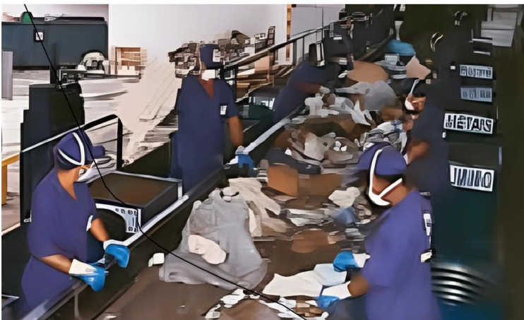
FIGURE 7: Detail of a manual selection of MSW recyclables in conveyor belt.
